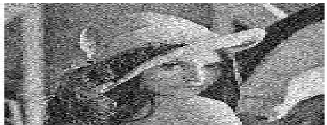
Figure 5:- An image corrupted by Gaussian noise of variance 0.01.
