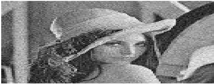
Figure 6:- Reconstructed image by the image which is corrupted by Gaussian noise of variance 0.01 using wavelet filter.
